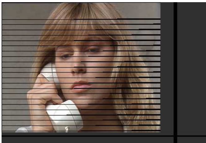
Figure 2.4: Image distortion when dot clock too high
