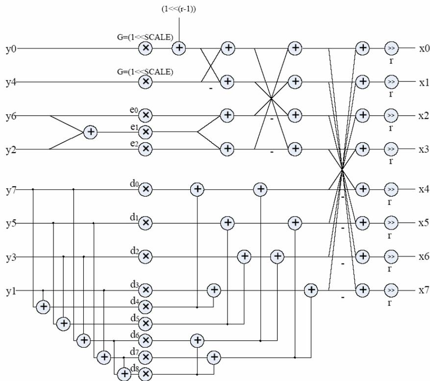
**Fig. 1.** IDCT Butterfly structure (including rounding)
